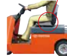
Floor Switch or Seat Switch detects the presence of the operator.
